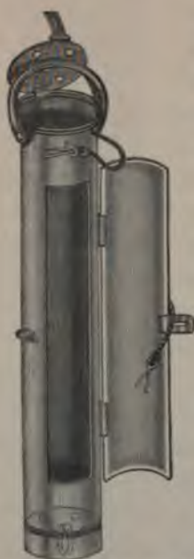
FIG. 54.—Copper case for protecting the Miller-Casella thermometer. The ends of the case above and below are perforated to allow a current of water to pass freely through.
